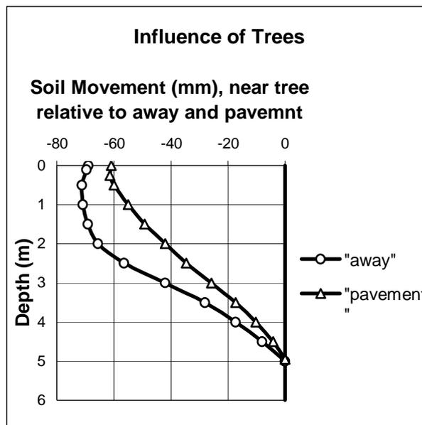
**Figure 5: Soil Movements Due To The Influence Of Street Tree**
