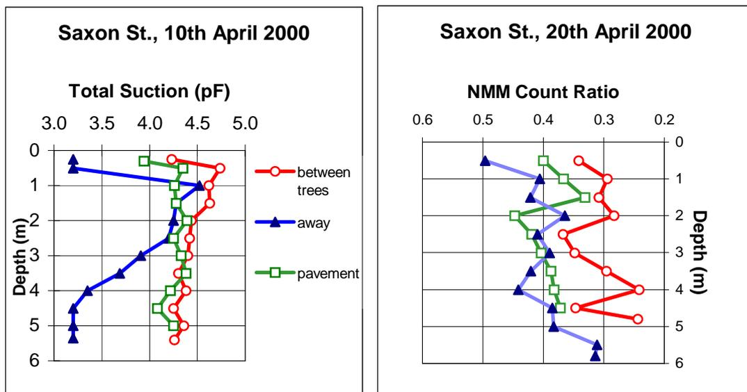
Figure 2: Soil suction profile and NMM count ratio profile, *Eucalyptus leucoxylon*
