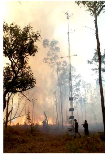
Figure 1 (a) Sapflow sensors measure the velocity of a heat pulse moving up the stem of trees. Eddy covariance towers have equipment to measure wind speed, wind direction, water vapour concentration and CO 2 concentration above canopies. From these measurements the flux of C to the canopy and water from the canopy can be calculated.
