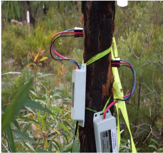
Figure 1 (a) Sapflow sensors measure the velocity of a heat pulse moving up the stem of trees. Eddy covariance towers have equipment to measure wind speed, wind direction, water vapour concentration and CO 2 concentration above canopies. From these measurements the flux of C to the canopy and water from the canopy can be calculated.
