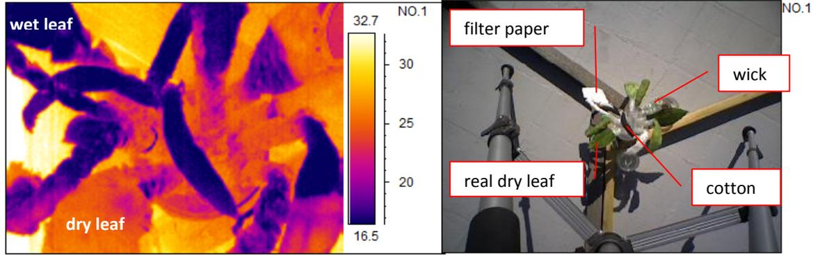
**Figure 1: Experimental setup in the laboratory for wet and dry leaf**
