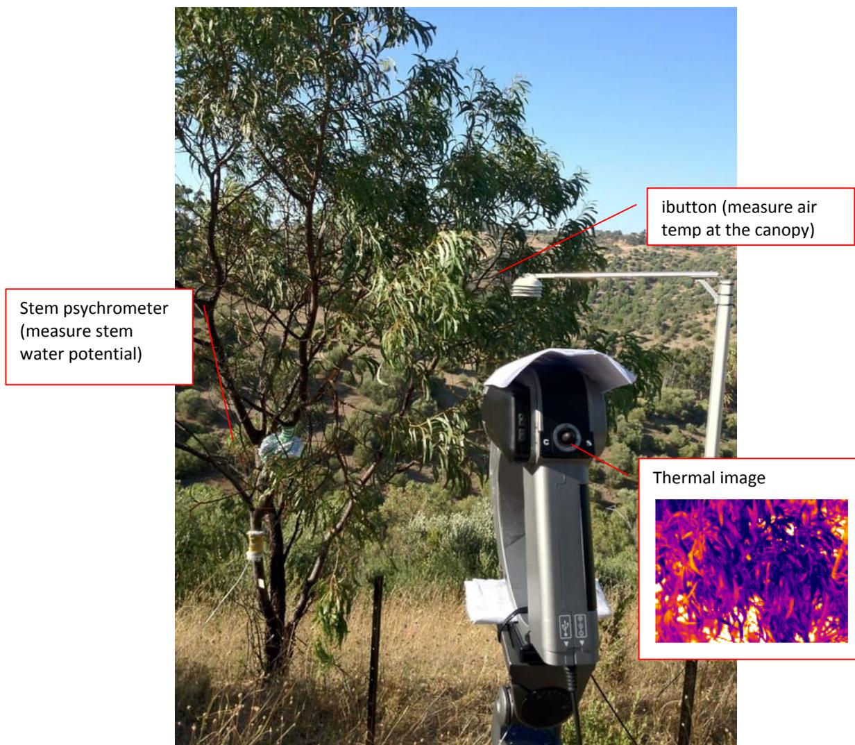
**Figure 2:** field experiment on Acacia tree with thermal imaging and stem psychrometer
