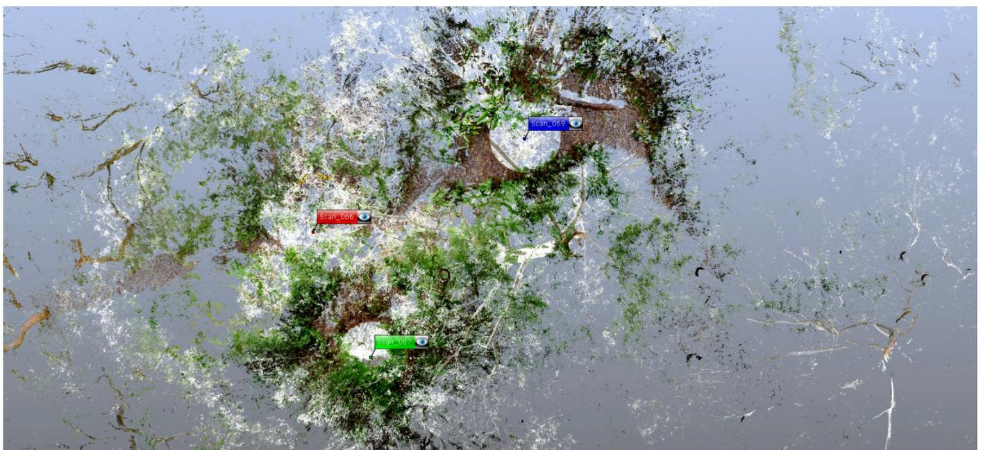
Point cloud acquired from FARO Laser Scanner Focus S150. Coloured point cloud acquired from three scan locations (blue, red, green) in plan view.
