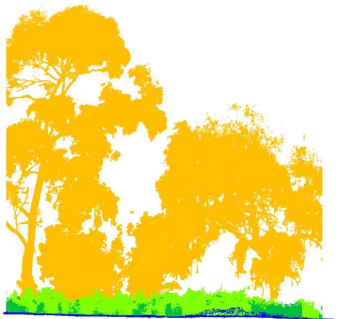
Point cloud acquired from Trimble TX-8 laser scanner. Classification of understorey vegetation according to three vegetation classes <1 m (Blue), 1-2 m (Green) & >2 m (Yellow).
