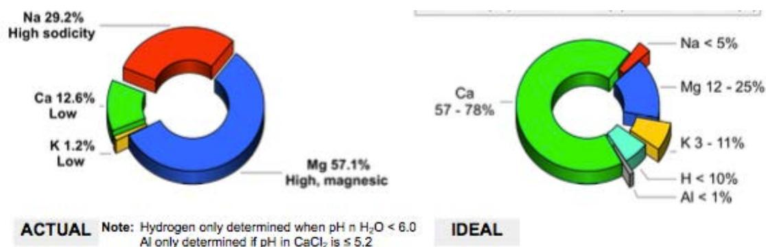
**Figure 2.** Graphical representation of tested vs. ideal cation balance (note ideal proportions are shown for topsoil – refer table 1).
