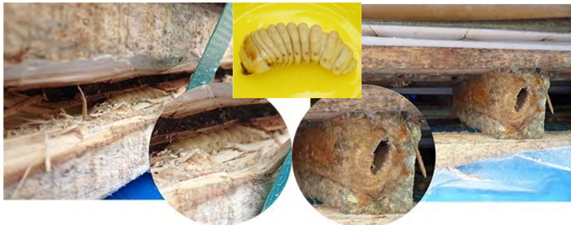
Figure 6. Timber pallet showing damage and longhorn larvae in situ and galleries within the wood (DA 2014)
