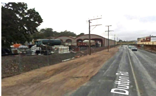
Figure 16. Verge compaction by vehicles can make soil impenetrable to roots (image: Google Streetview 2008)
