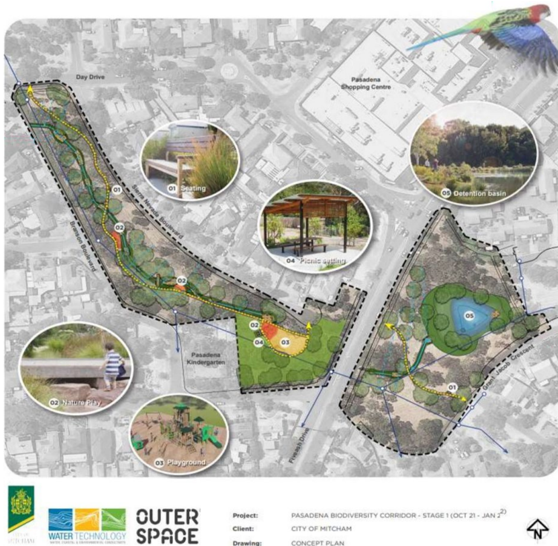
Figure 3: Concept plan of Pasadena Biodiversity Corridor Stage 1 (Oct 21 – Jan 22) with swale and detention basin layout.
